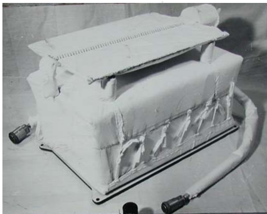
Thermostable electronic block with MLI
