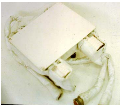
Electronic block with isothermal electronic card
