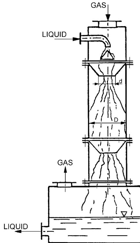
Fig. 1. Scheme of the spray - cascade co-current absorber.
