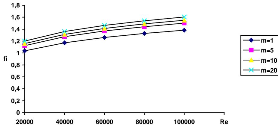
Fig. 4. Effect of gas Reynolds number and two-phase flow number on enhancement factor  $\phi_v$  for confusor K3 with swirl plate and profiled inside surface.
