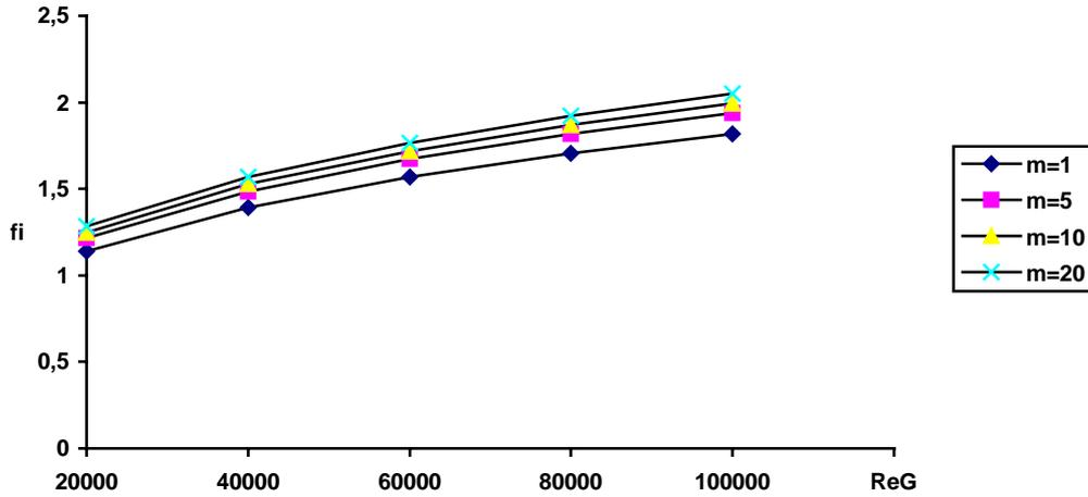
Fig. 3. Effect of gas Reynolds number and two-phase flow number on enhancement factor  $\phi_v$  for confusor K2 with swirl plate.
