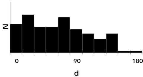
Fig. 4. Drop-size histogram for pressure-swirl atomizer ( $\hat{d}=125\mu\text{m}$ ).
