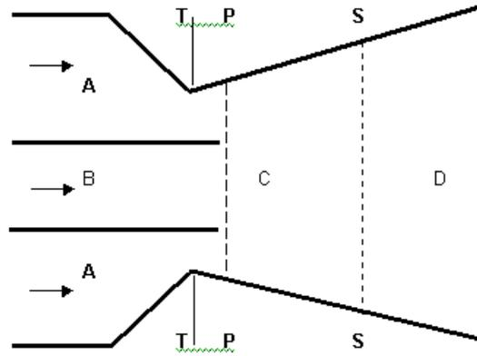
**Fig. 2.** Scheme of the gas atomizer without central body.
