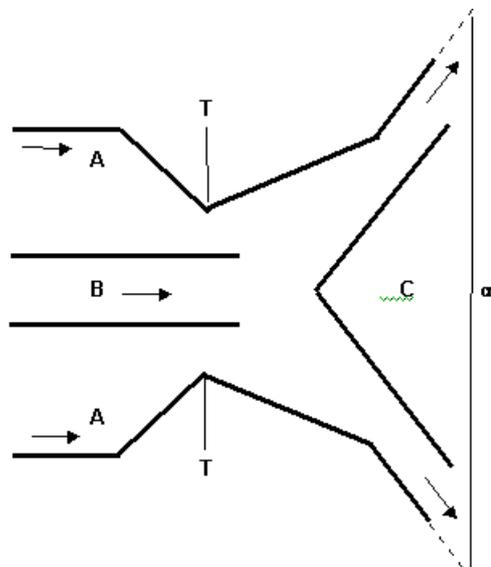
**Fig. 1b.** Scheme of the gas atomizer with a central body.
