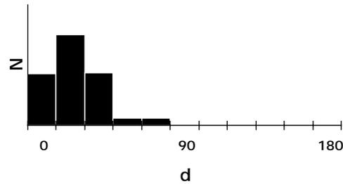
Fig. 5. Drop-size histogram for gas atomizer ( $\hat{d}=61\mu\text{m}$ ).
