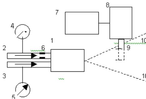
**Fig. 3.** Scheme of the drop-size measurement system.
