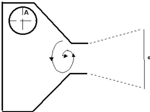
**Fig. 1a.** Scheme of the pressure-swirl atomizer.
