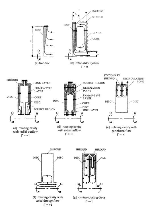
Fig. 1 Schematic diagram of rotating-disc systems
