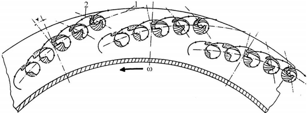
Fig. 2 The image of flow in the second stage – formation of secondary vortices:
