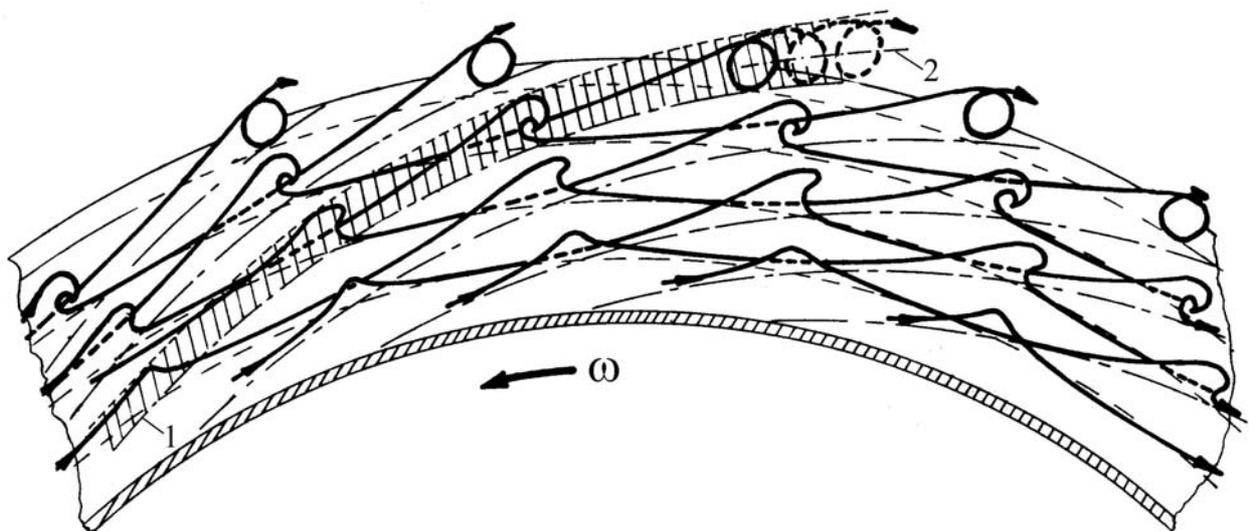
Fig. 1 The image of flow in the first stage - transition from wavy to vortex form:
