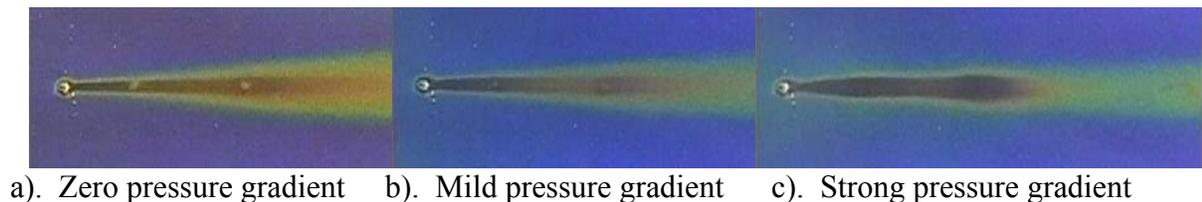
**Fig. 2.** TSLC results for the turbulent wedge under zero, mild and strong pressure gradients respectively.
