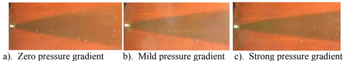
**Fig. 1.** SSLC results for the turbulent wedge under zero, mild and strong pressure gradients respectively.
