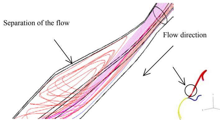
Figure 2: Streamlines at the stenosis (steady case).
