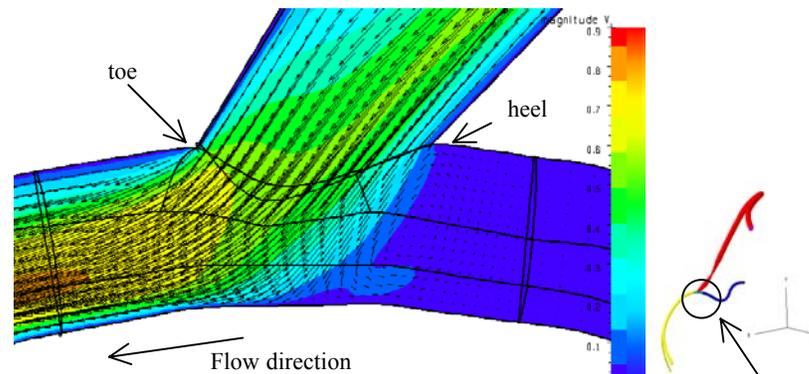
**Figure 3: Velocity field and magnitude (range 0-0.9 m/s) at the anastomosis (plane in the middle of the vessel).**
