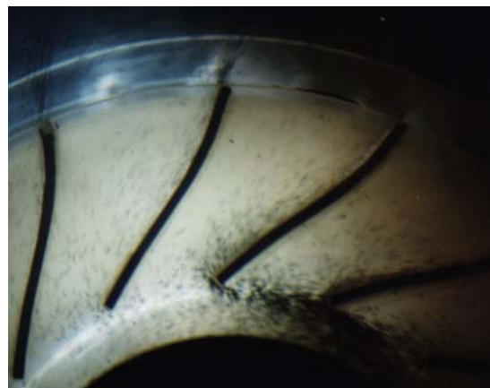
Figure 3: Particle trajectory in backward straight impeller
