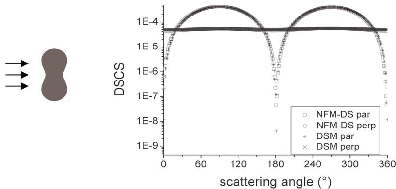
Figure 2: Comparison of light scattering patterns calculated by NFM-DS and DSM. Particle shape is a Cassini-oval based peanut as shown in Fig. 1, particle length is 100nm. Wavelength is 478nm, incident angle is  $90^\circ$  to rotational axis; therefore forward scattering can be observed at  $90^\circ$ . Refractive index is  $0.13-2.729i$ .
