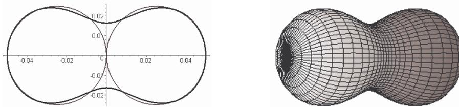
Figure 1: Cassini-oval based shape model; two-dimensional compared to two equi-volumed spheres (left) and the corresponding three-dimensional model (right).  $a = 0.0340625$ ,  $b = 0.0365625$ ,  $c = 1.236$ ; the diameter of the spheres is 50nm. Overall particle size is 100nm.
