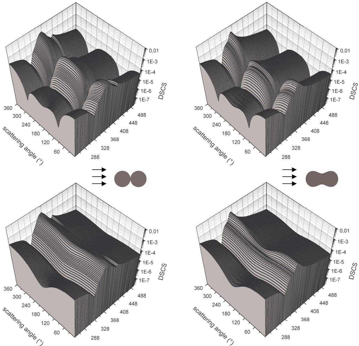
Figure 3: Spectral analysis of two spheres (left) and an equi-volume Cassini-oval based peanut (right) as shown in Fig. 1. Particle length is 100nm. Wavelength-range is from 250nm to 500nm; direction of incident light is along rotational axis. Upper diagrams show parallel, lower diagrams show perpendicular polarization.
