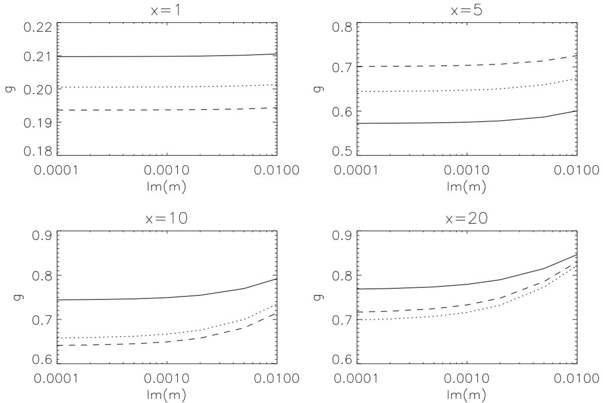
Figure 1: Dependence of the asymmetry parameter  $g$  on the imaginary part of the refractive index,  $\text{Im}(m)$ , for spheres (solid line), equiprobable shape distribution (dotted line), and weighed shape distribution (dashed line).
