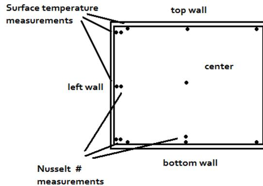
Figure 2. Positions of the thermocouples
