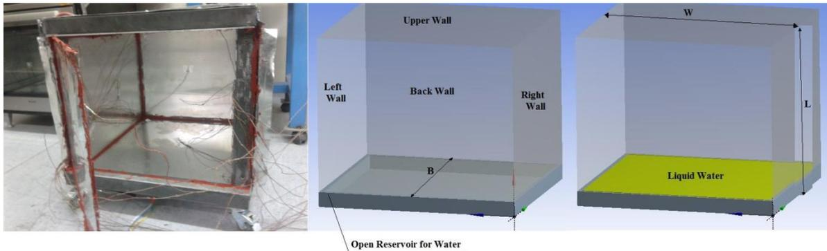
Figure 1. Schematics of Experimental Setup
