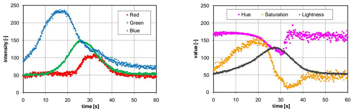
Figure 1: Temporal TLC signals in RGB (left) and HSL (right) color coding during a transient test
