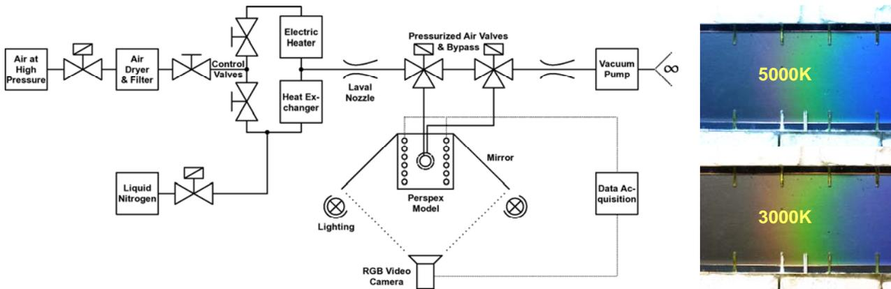
Figure 3: Experimental Setup for Transient Heat Transfer Experiments in Complex Cooling Schemes (left) and impact of color temperature of lighting on TLC observation (right)
