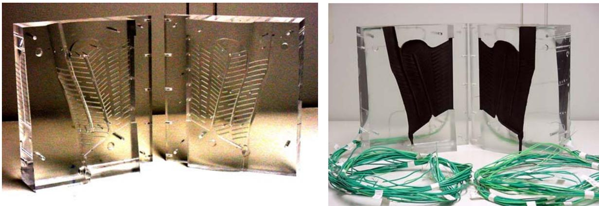
Figure 2: Full cooling scheme model parts for a gas turbine blade as machined from Perspex (left), coated and instrumented model parts (right).
