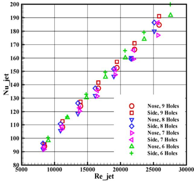
Fig. 2 Impingement jet Nusselt number versus jet Reynolds number on the nose and side walls for cases of 9, 8, 7 and 6 cross-over holes.
