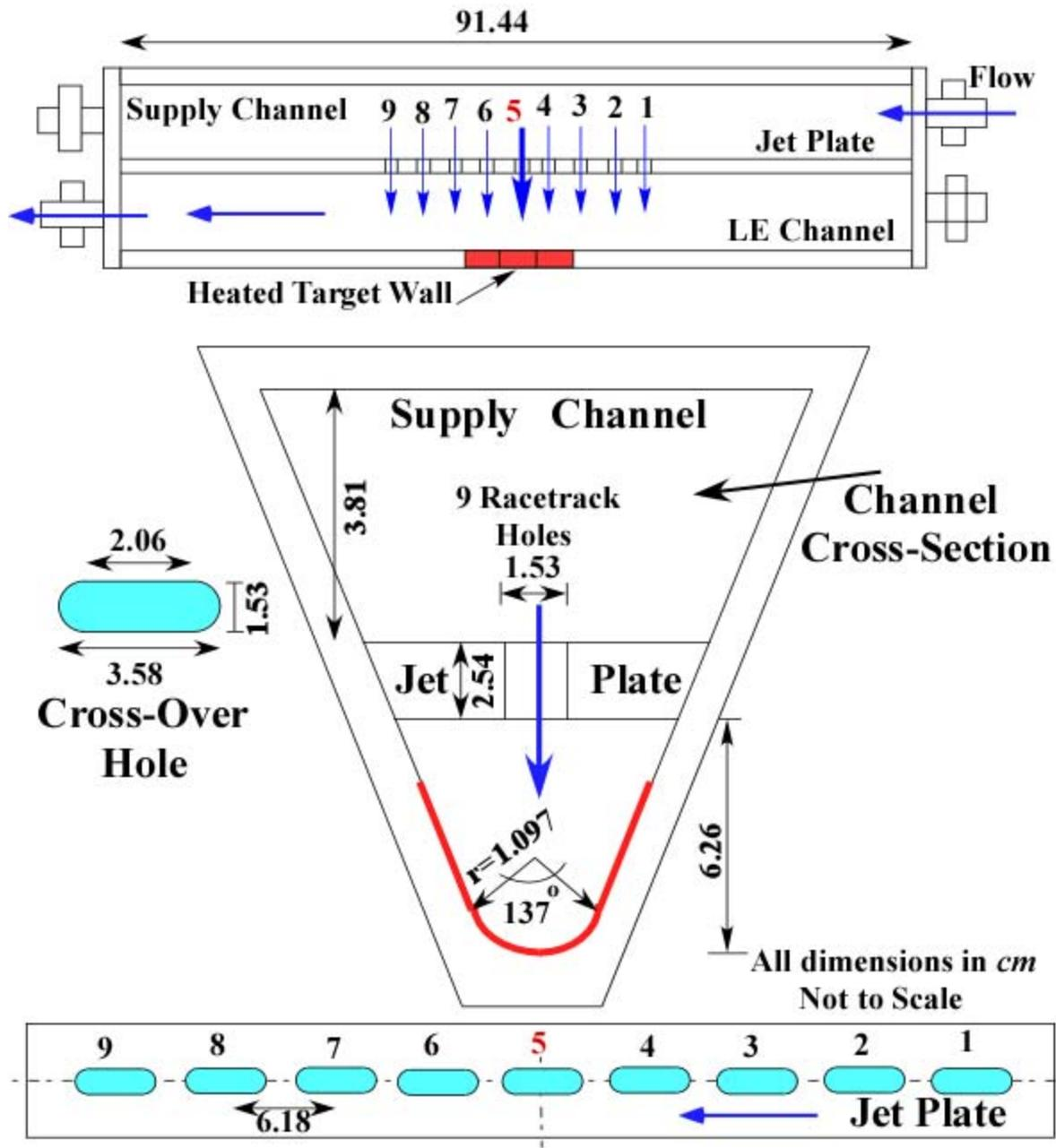
Fig. 1 Schematics of the rig.
