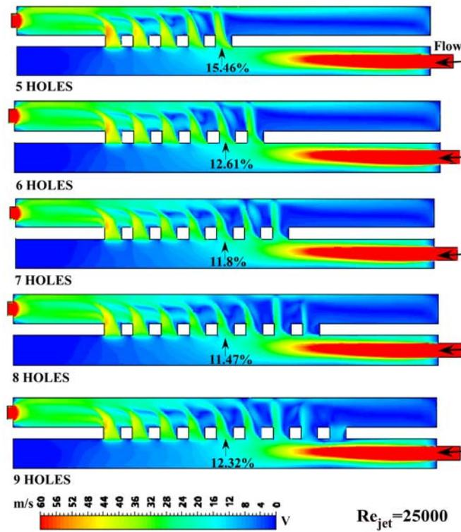
Fig. 4 CFD contours of velocity magnitudes for cases of 9, 8, 7, 6 and 5 cross-over holes.
