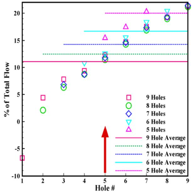
Fig. 3 Percentage of total flow through each cross-over hole for cases of 9, 8, 7, 6 and 5 cross-over holes.
