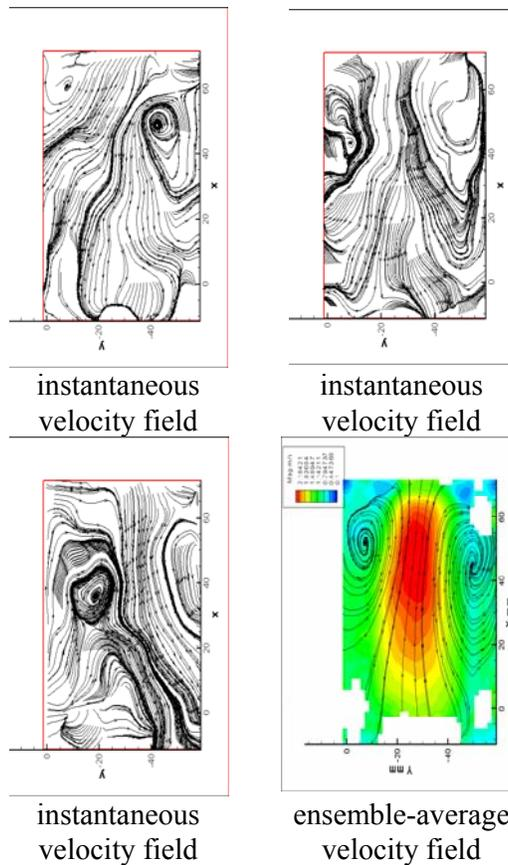
Figure 4 instantaneous velocity field and ensemble-average velocity field
