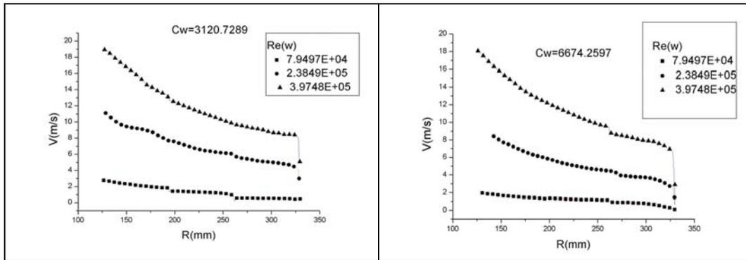
Figure 3 Radial distributions of the tangential velocity
