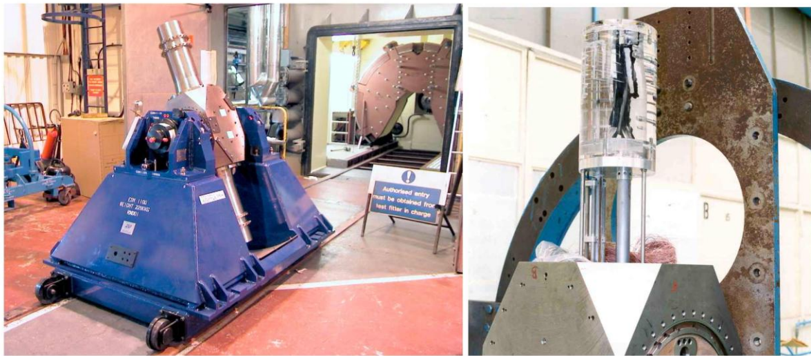
Figure 1 The Rotating Heat Transfer Rig used by Rolls-Royce to study the effect of rotation on blade cooling flows.
