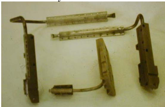
Radiative cooling system for mission “Venera-Galey”
