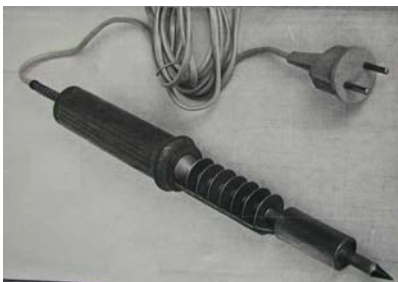
Soldering tool on the base of VCHP Temperature level 258 °C \pm 2
