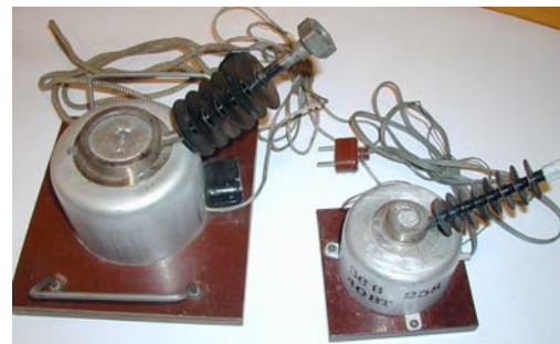
Soldering bathes for tin-lead alloys on the base of VCHP. Temperature level is 258 °C \pm 2
