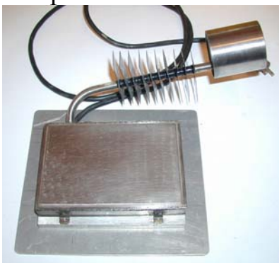
Thermostable plate for tin-lead alloys on the base of VCHP Temperature level 220 °C \pm 2
