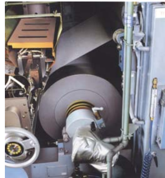
Cylindrical heat pipe for providing homogeneous surface roller temperature of 29 °C for offset printing, extrusion laminators
