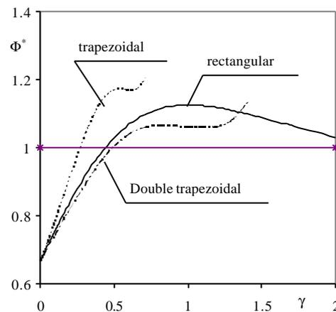
Fig. 1 – The parameter  $\Phi^*$  defined by Eq.(1) as function of the micro-channel cross-section geometry.
