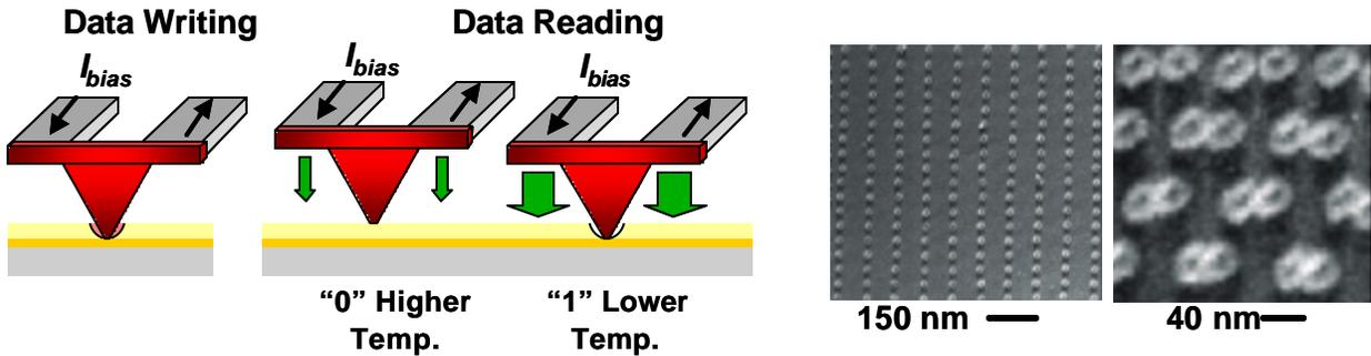
Fig. 1. Schematic of the thermomechanical data storage process and images of the resulting data bits (1).
