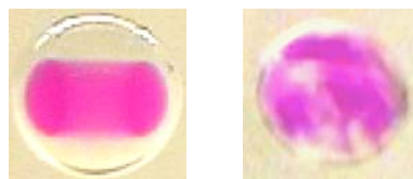
Fig. 1: Neutralisation front of acetic acid with Marangoni convection (right) and without Marangoni convection (left)
