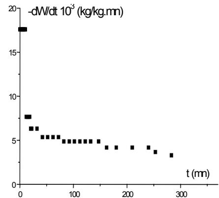
Figure 3: Graph of the drying velocity
