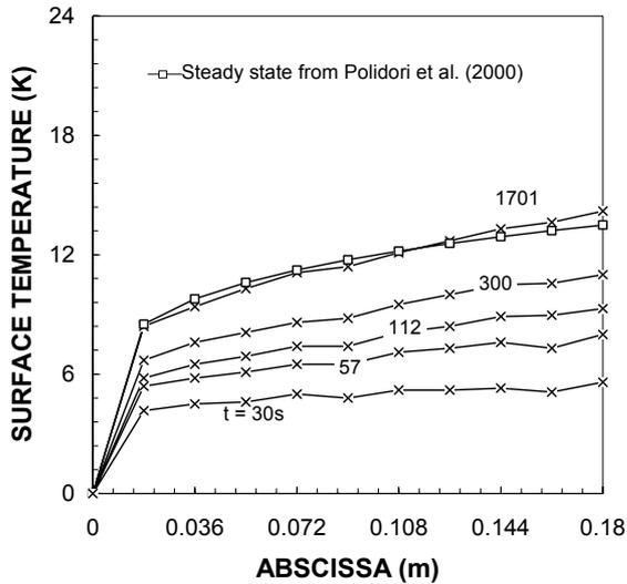
Figure 1 : Streamwise temperature distribution along the smooth wall (1)
