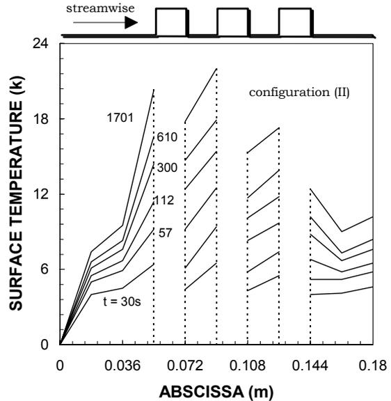
Figure 2 : Streamwise temperature distribution along the ribbed wall in the configuration (II).
