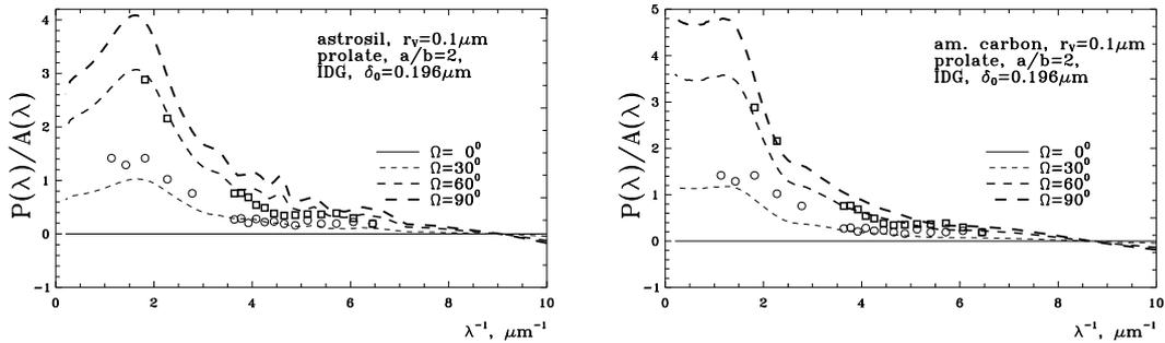
Figure 3: Wavelength dependence of polarizing efficiency for homogeneous rotating spheroidal particles of astronomical silicate and amorphous carbon. The effect of variations of particle composition and direction of alignment is illustrated. The open circles and squares show the observational data for stars HD 24263 and HD 99264, respectively.
