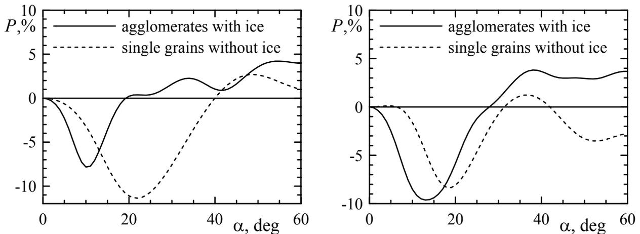
Figure 2: Phase curves of degree of linear polarization of agglomerates covered by ice and single constituent grains. Left panel: pure silicate grains. Right panel: grains with a silicate-core plus organic-mantle structure.
