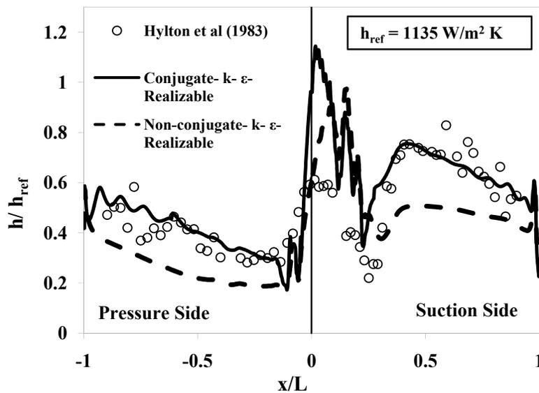
Fig 1. Heat transfer coefficient along the blade surface
