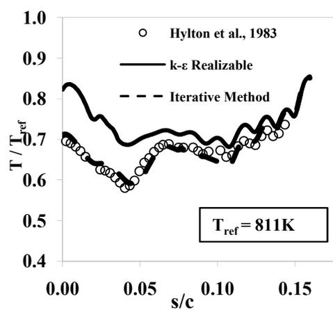
Fig 3. Temperature along the suction surface
