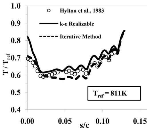
Fig 2. Temperature along the pressure surface
