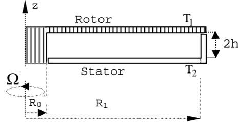
Figure 1. Schematic picture of the rotor/stator cavity.
