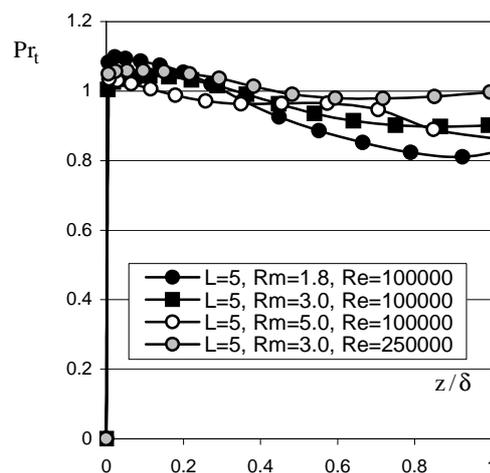
Figure 5. Axial distributions of the turbulent Prandtl numbers  $Pr_t = (-\overline{v'w'}/\partial v/\partial z)/(\overline{\Theta'w'}/\partial \Theta/\partial z)$  obtained in the middle section of cavities.
