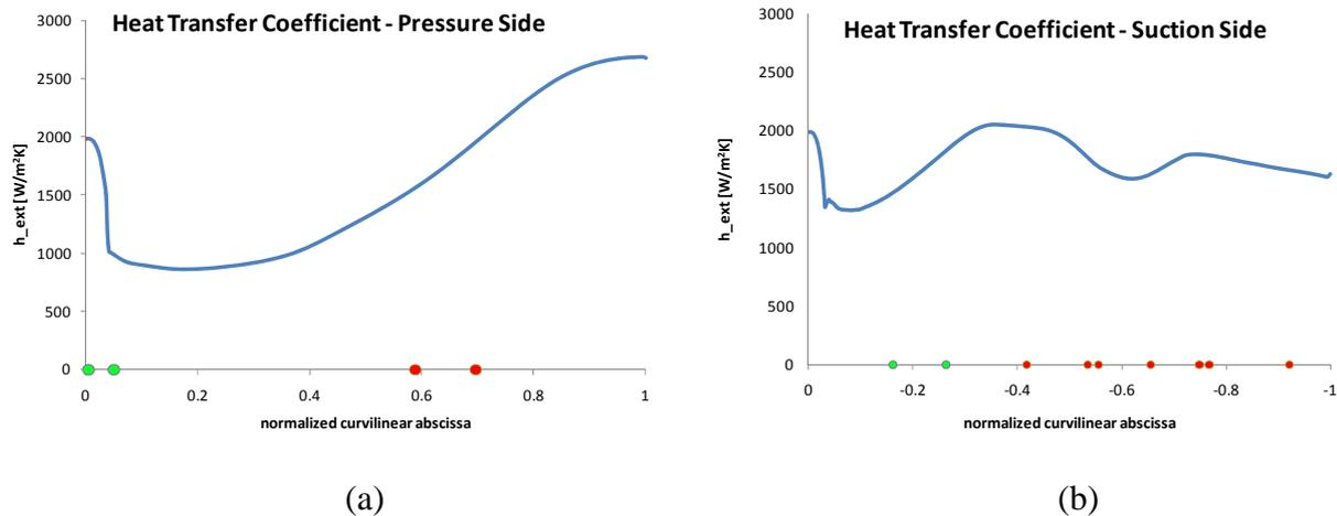
Figure 3. Convective heat transfer coefficients vs. normalized curvilinear abscissa:
