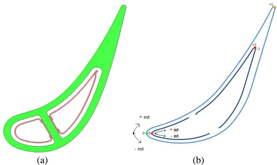
Figure 1. Geometry of the (a) midplane stator nozzle, and (b) normalized curvilinear abscissas, Pressure and Suction side starting from the leading edge
