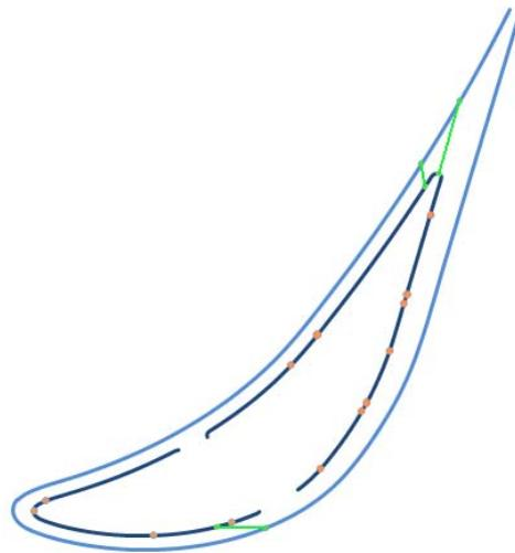
Figure 2. An example of an optimized configuration with impingement and film cooling holes.
