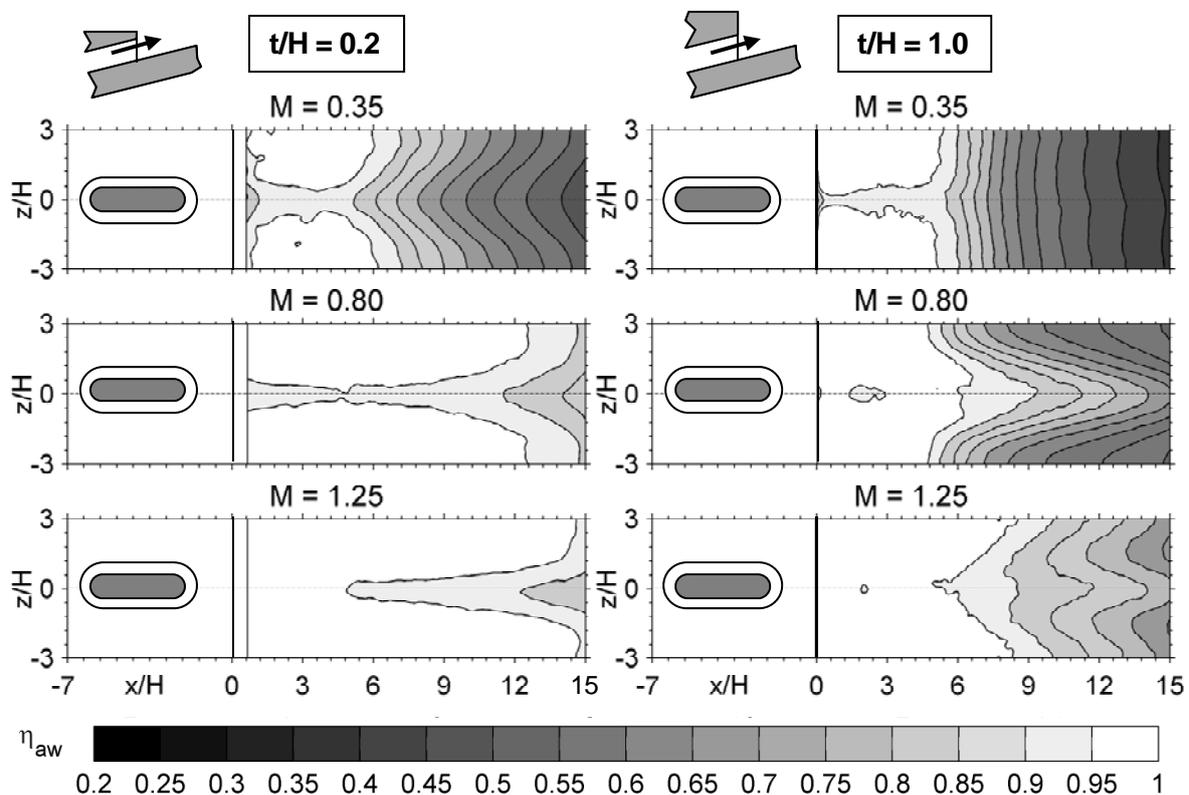
Figure 2. Contours of local film cooling effectiveness downstream of the ejection slot at different blowing ratios for two different lip thicknesses
