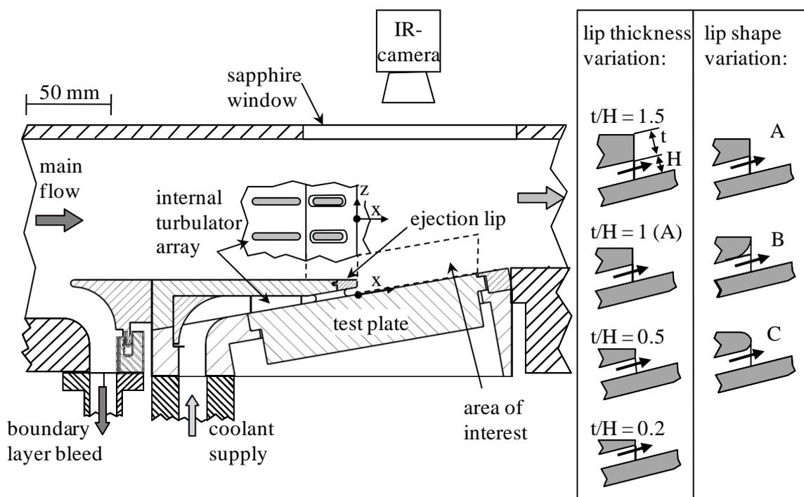
Figure 1. Generic test section for trailing film cooling experiments with varying ejection lip geometry
