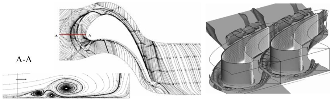
Figure 2. Secondary flow structure in the NASA GRC transonic blade cascade after RANS simulation by Levchenya & Smirnov [2007]
