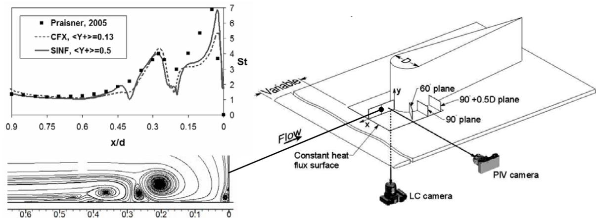
Figure 3. Experimental configuration of Praisner & Smith [2006] and results of RANS simulation of the horse shoe vortex system and endwall heat transfer near the airfoil LE [Levchenya et al. 2009]
