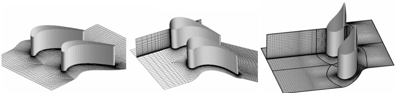
Figure 1. Geometry and typical computational grids used for numerical simulation of 3D flow and heat transfer in test linear cascades: (left) Langston subsonic blade cascade, (mid) NASA GRC transonic blade cascade, and (right) Virginia Tech vane cascade
